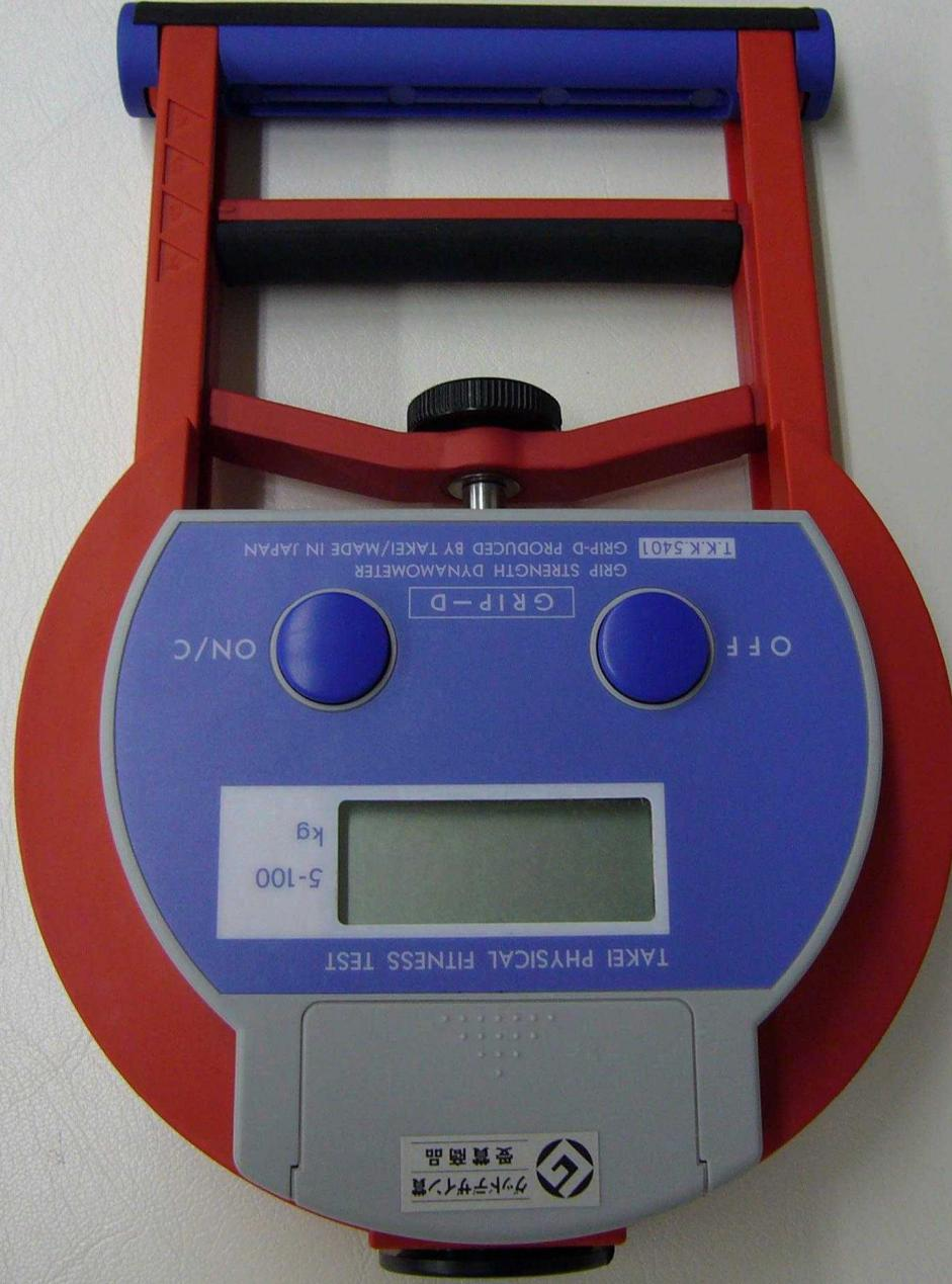
T.K.K.5401 GRIP STRENGTH DYNAMOMETER GRIP-D PRODUCED BY TAKEI/MADE IN JAPAN
